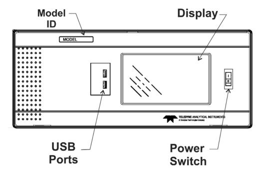
Figure 3-1: Front Panel Layout
